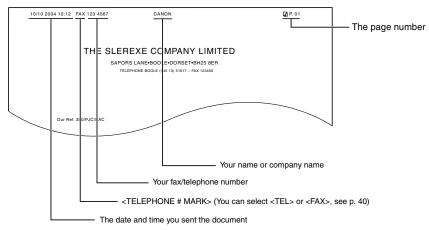
The top line includes the name of the receiving party if you send the document using one-touch speed dialling or coded speed dialling and you registered the party's name.
